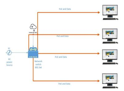
User safe – PoE (power over Ethernet) is covered by the low voltage directive and is inherently safe to use. 100W (IEEE's 802.3bt++) Power Injector
